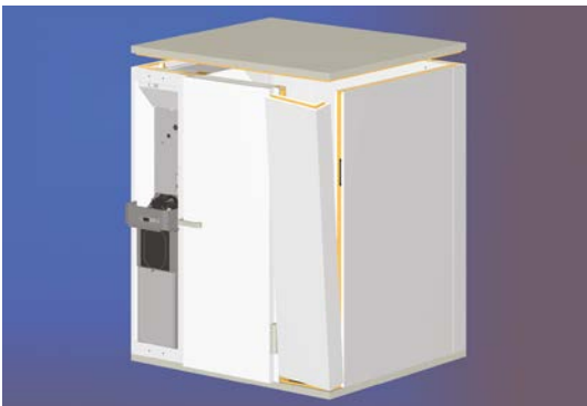
Figure 10. The assembly of the corner and roof elements
