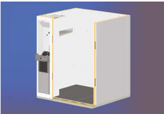
Figure 9. The assembly of the wall panels
